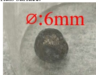
Figure 3: Metallic Spheroid Produced in Electro-Deoxidation
